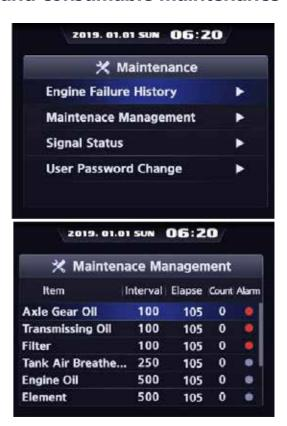
Engine failure can be checked in clusters without the need for a separate engine diagnostic tool, and the parts to be replaced are displayed in the cluster during operation when the replacement timing of all consumables requiring periodic maintenance is set in the cluster.
