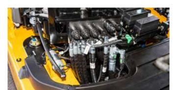
The load-sensing MCV has a very low internal leakage, resulting in a dramatic reduction of the amount of natural settlement (change in position due to its own weight) of the lift and tilt lines. Along with this feature, the Lift Emergency Lowering Screw and a Descending Speed Adjustable Regulator of the MCV reduce the maintenance frequency and downtime.
