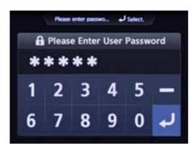
To prevent theft, breakdown, and safety accidents when the equipment is not in use that may occur when unauthorized people try to use the equipment without the administrator's permission, the operator's passcode can be set on the cluster to restrict the operation of the equipment.
