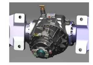
The negative-type auto parking brake operates automatically when power is cut off in order to prevent safety accidents caused by human error, like not operating the parking brake lever, and backsliding is prevented upon restarting on a slide with the Hill Start Assist Control (HAC).
