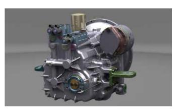
HDX's transmission and drive axle transmission, which have improved durability and practicality, increased clutch pack power transmission capability by 25% and T/M oil quantity, considering high-load working conditions. The reverse gear with a low frequency of use is made into one gear, and to the forward gear consisting of two steps is applied an automatic transmission system for increased practicality and convenience.
