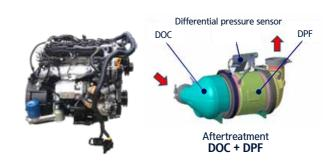
The HMC D4CC engine with optimized displacement for a forklift comprises an electronic EGR valve, a common rail, Variable Geometry Turbo-charger (VGT) with an excellent boosting effect, and aftertreatment (DOC + DPF) device. It also meets the stricter EU Stage 5 regulations.
