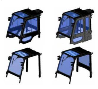
From cabin with air conditioning and heater (1Door / 2Door) to partial cabin(Front&Top, Front&Top&Rear). Various cabin options are available.
