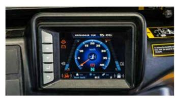
In the new cluster, the size and characteristics of the symbols have been adjusted for better visibility of driving information and safety warnings, and MCU functions are integrated to simplify parts.
