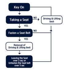
The seat belt interlock system, which restricts forklift operation when the seat belt - wearing order is not observed or the operator releases the belt while driving, prevents operator injury from safety accidents that may occur when the seat belt is not fastened.
