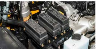
The fuses and relays that are vulnerable to contamination are placed inside a box with enhanced waterproof and dustproof functions, and the box itself is placed inside the engine room to reduce maintenance downtime.
