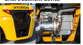
To eliminate the inconvenience of removing the counterweight to inspect the aftertreatment device inside the weight, the opening of the counterweight has been expanded to the maximum extent possible.
