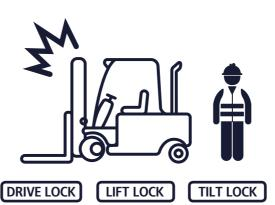
The OPSS that restricts driving, lifting, and tilting kicks in when the operator leaves the driver's seat in order to prevent safety accidents. It is simultaneously operated with the auto parking brake to create a safer workplace.
